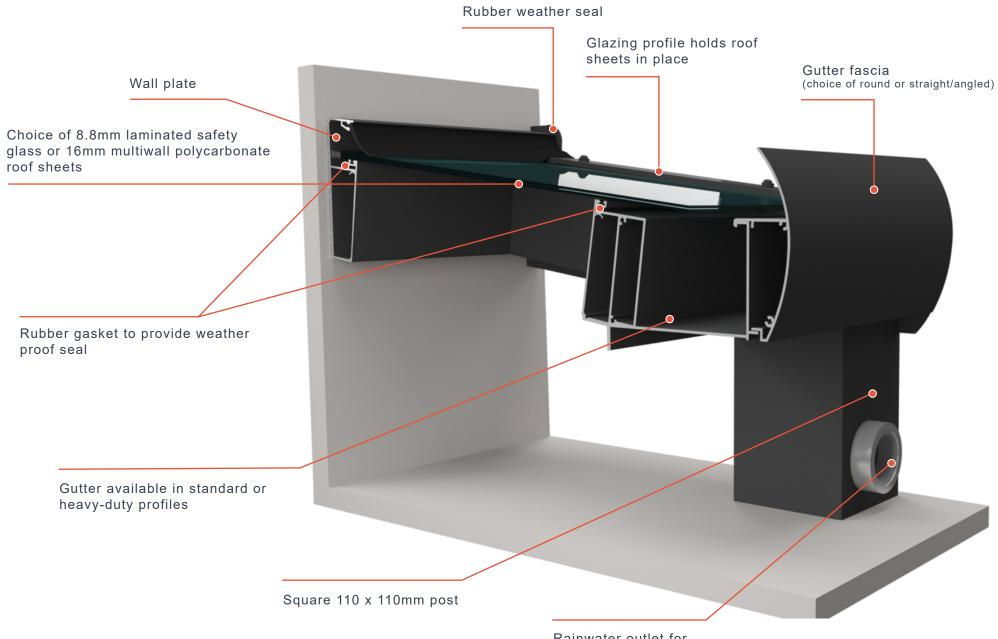
Rainwater outlet for integral drainage
